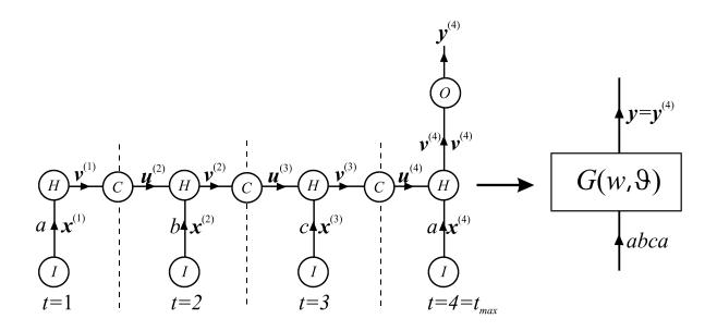
Unfolded Elman's network is of the standard "feed forward" type that can be simply adapted by the "back propagation" method.
