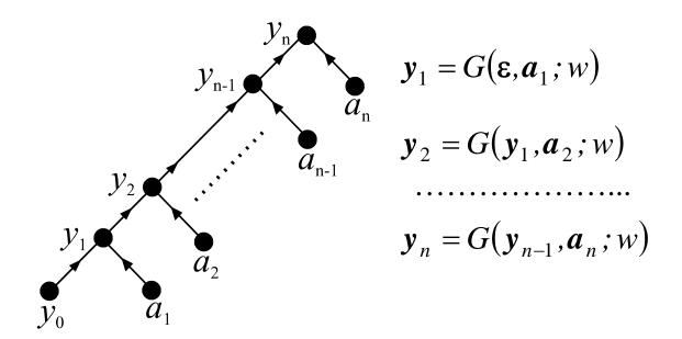
A final vector  $\mathbf{y}_n$  represents a mapping of the string  $\alpha = (a_1 a_2 ... a_n) \in A^*$  onto a p-dimensional real vector  $\mathbf{y} = (y_1, y_2, ..., y_p) \in (0,1)^p$
