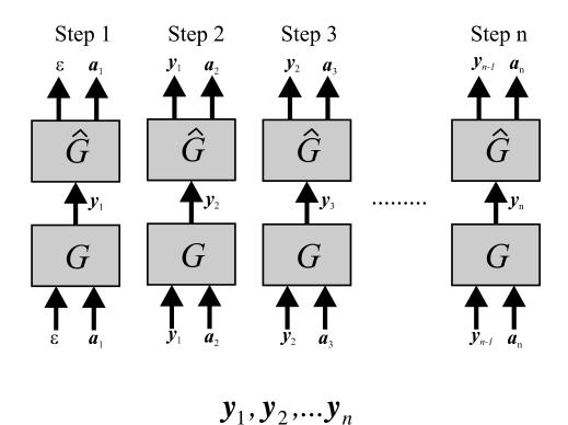
The last vector  $y_n$  is a final output from the RAAM mapping  $G_{tot}$ . If this mapping is auto-associative (i.e. input and output are equal), then  $y_n$  is a vector code of the string  $\alpha$ . Formally
