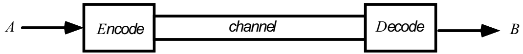
Fig. 4. The standard communication channel (“the information theorist’s coat of arms”). The source (Alice) produces information which is manipulated (‘encoded’) and then sent over the channel. At the receiver (Bob) the received values are ‘decoded’ and the information thus extracted.
